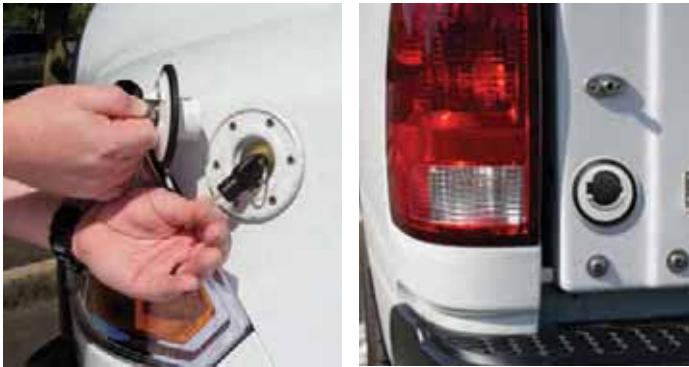
Permanently-mounted key storage tube keeps keys where you need them.
